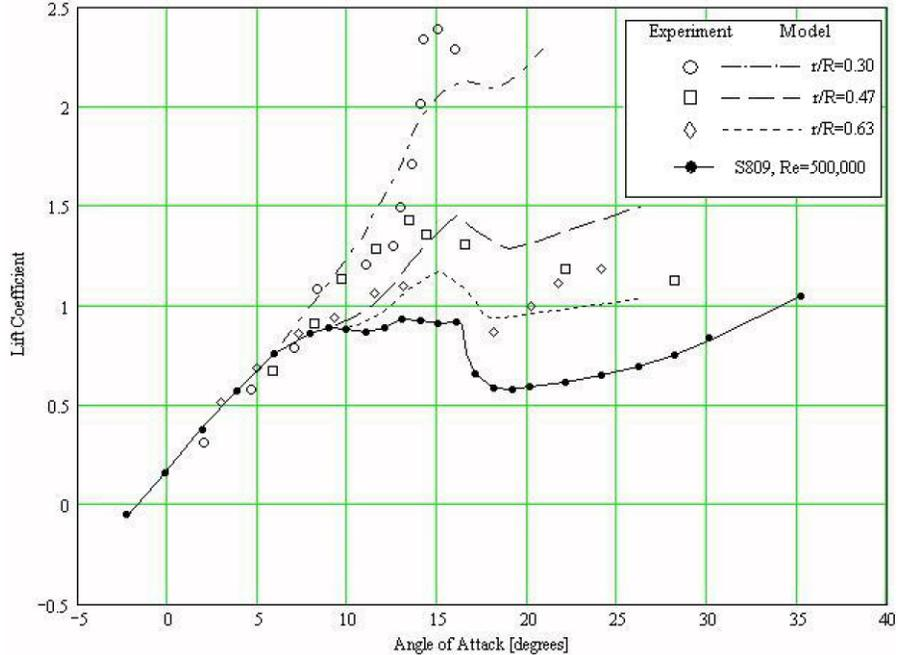
Fig.4. Effect of the radial position on the lift coefficient
