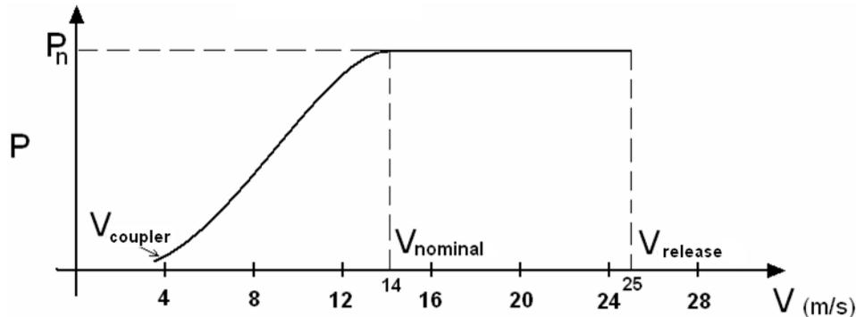
Figure 1. A power curve of a wind turbine with indicative numerical values
