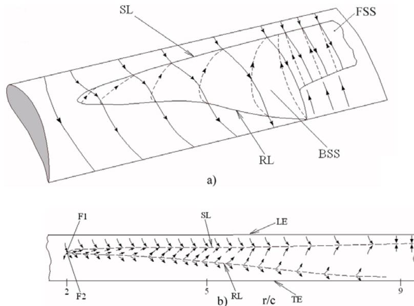
Figure 3. Topological structures of separation on rotating blade: a) types of separation surface; b) separation/reattachment.
