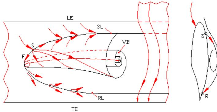
Figure 2. Formation of the standing vortex in the radial direction
