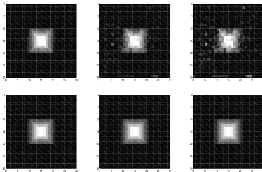
Fig. 6. Images reconstructed from noisy (inconsistent) data with the algorithms: CK (top row), CKERP (bottom row), for different values of parameter  $\epsilon$ : 10 (left column), 30 (middle column), 50 (right column).
