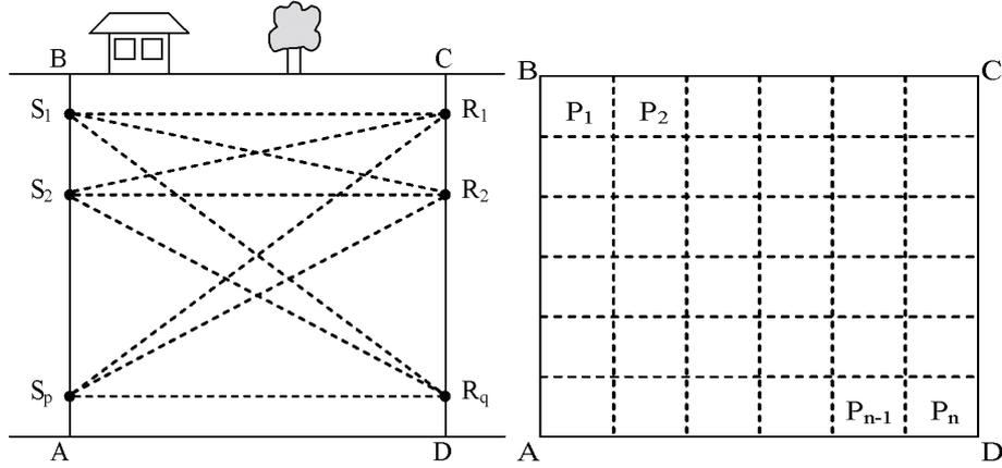
Fig. 1. (Left) Measurement setup in electromagnetic geotomography; (Right) Discretization of the scanned area.
