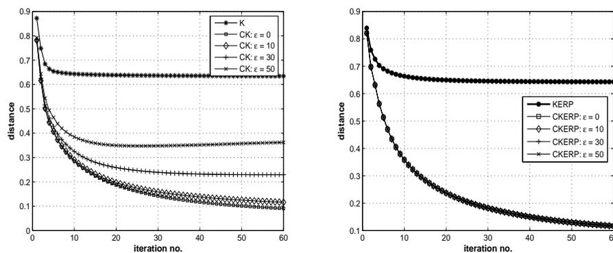
Fig. 7. Normalized Euclidean distances between the exact images ( $x_{\text{exact}}$ ) and the image reconstructed with the algorithms: CK (top), CKERP (bottom).
