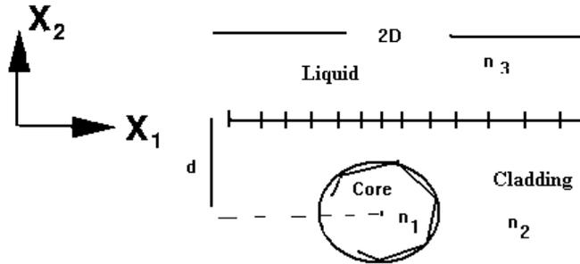
Fig. 3. Approximated interfaces of the optical half coupler.
