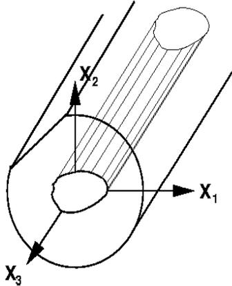
Fig. 1. An optical half coupler.
