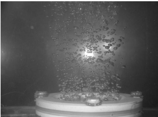
This regime is obtained for  $Q < Q_s$  air flow rates and the formed bubbles are isolated and have a uniform size (fig. 1).
