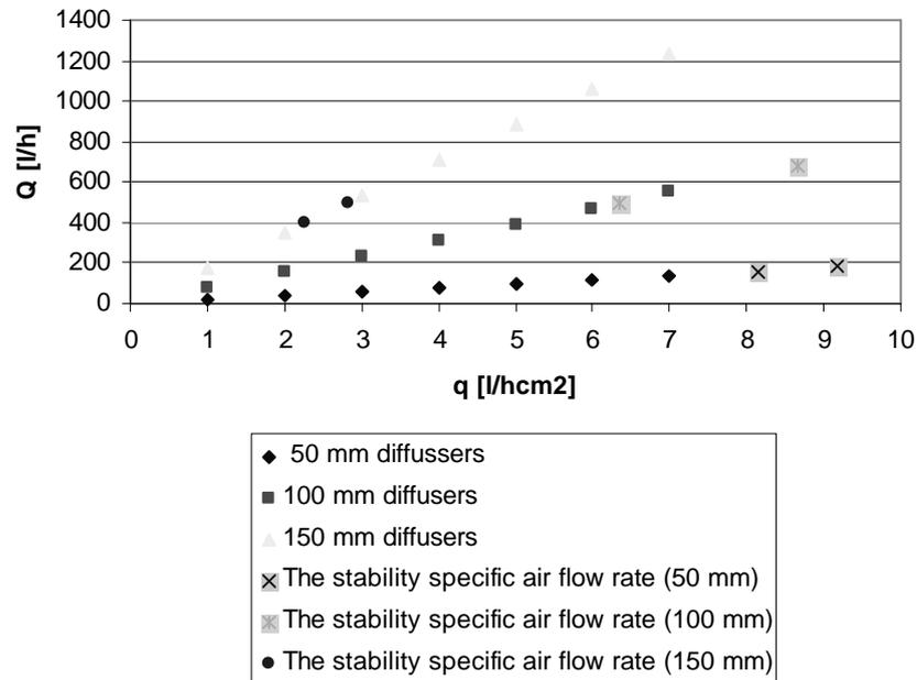
Fig. 4, The stability specific air flow rates for the tested porous diffusers
