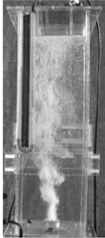
Fig. 7, *The bubbles column aspect at  $Q=400$  l/h*      Fig. 8, *The bubbles column aspect at  $Q=450$  l/h*
