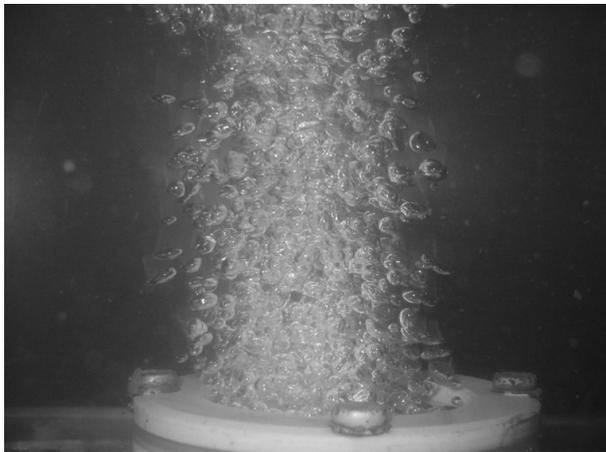
Fig.3, Bubbles emission aspect in turbulent regime for a ceramic porous diffuser  $F = 50 \text{ mm}$
